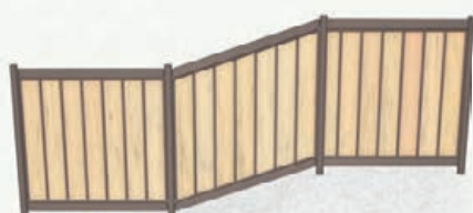
FOLLOWING THE TERRAIN OBLIQUELY
