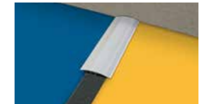
ADAPTABLE TRANSITION STRIPS Aluminium adaptable transition strip Compensating up to 14mm difference in level 1 box of 10 pcs - 27lm 41mm high x 2700mm long
